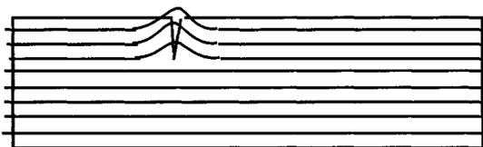
**Fig. 25.25** Schematic representation of the magnetic lines of flux in a ferromagnetic metal near a flaw. Small magnetic particles are attracted to the leakage field associated with the flaw.
